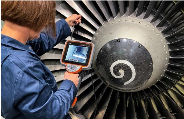
An operator using a Mentor Visual iQ+ video borescope to inspect a GE engine
