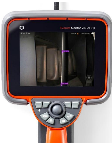
Mentor Visual iQ+ video borescope with Gas Power-assist 5.0 analytic showing dent indications on the leading edge of a high-pressure compressor blade
